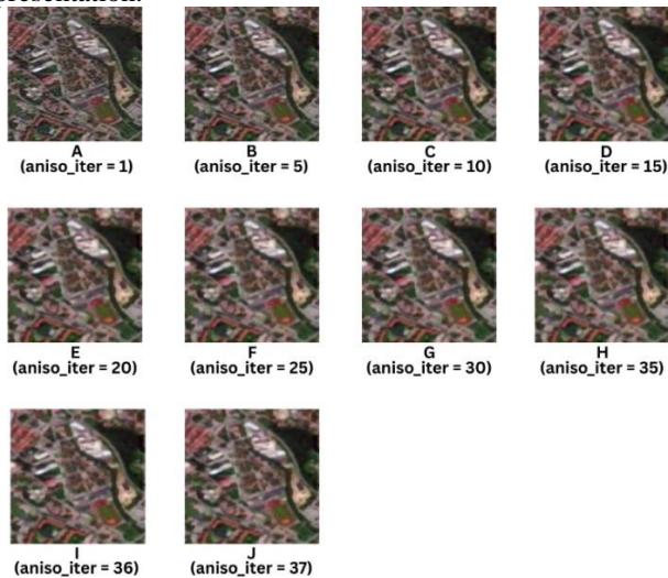
Fig. 16. Fusion quality variation across anisotropic diffusion iterations (Dataset E).
